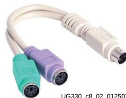
Figure 8-6: Example PS/2 Y-Splitter Cable
