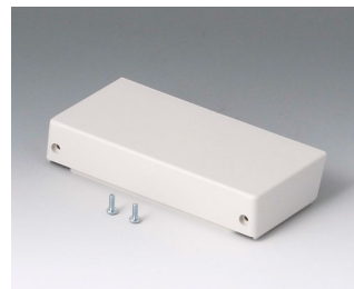
B4016417 Lid M closed, flat ABS (UL 94 HB) off-white RAL 9002 5.28"x2.44"x0.94"
