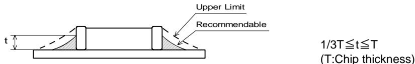
Accordingly increasing the solder volume, the mechanical stress to product is also increased. Exceeding solder volume may cause the failure of mechanical or electrical performance.
