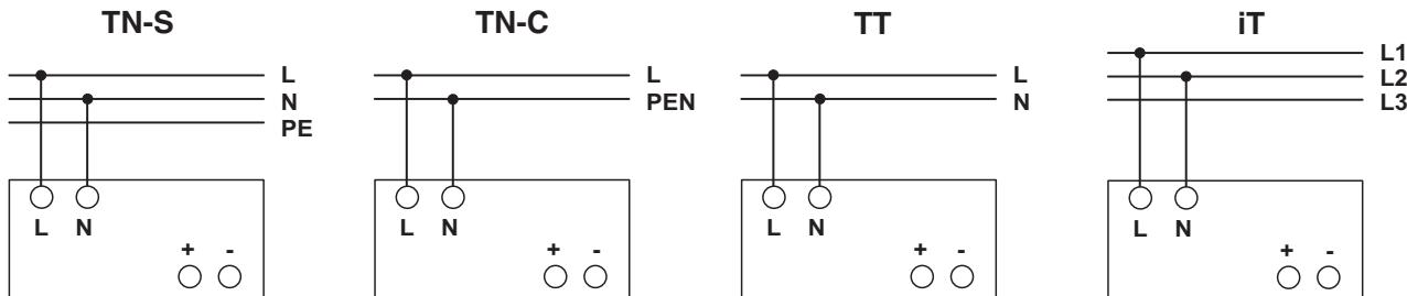
The 100...240 V AC connection is made using the L and N screw connections.
