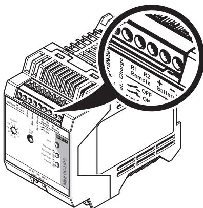
The device has a remote shutdown with a UPS function for deliberate shutdown. Remote shutdown must be deactivated for the device to switch over to the buffer mode in the event of a supply voltage failure.
