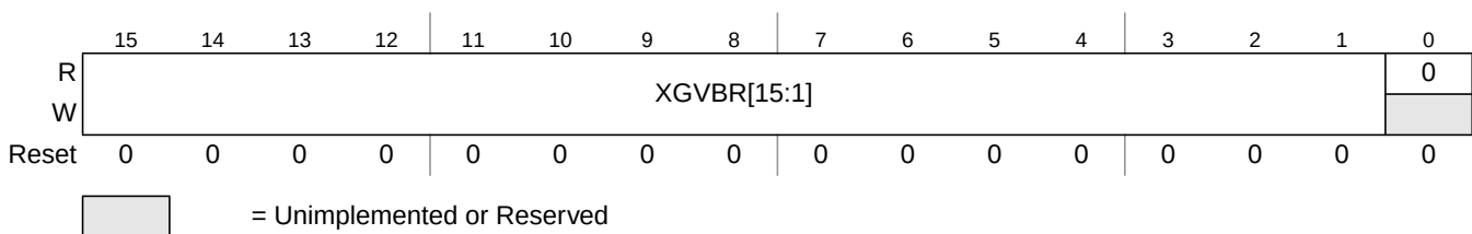
Figure 6-5. XGATE Vector Base Address Register (XGVBR)
