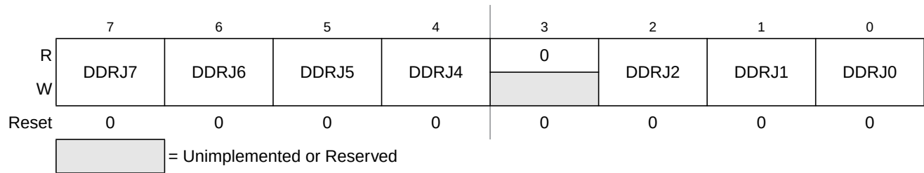
Figure 22-58. Port J Data Direction Register (DDRJ)
