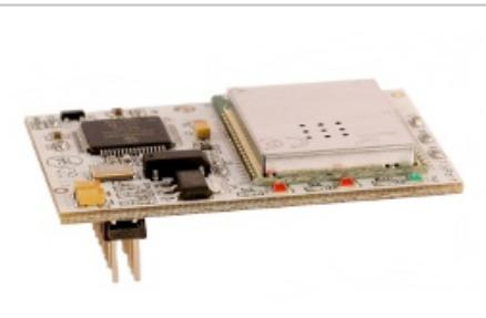
FLYPORT is powered by openPicus framework based on FreeRTOS. The free IDE allows to create applications, to import web pages and to compile and download code to the module.
