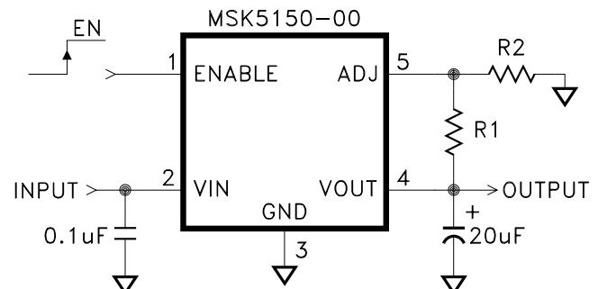
$$V_{OUT} = 1.240V \times [1 + (R_1/R_2)]$$
