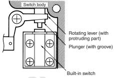
Be sure to check the mechanical lock and solenoid release functions when mounting the D4BL.
