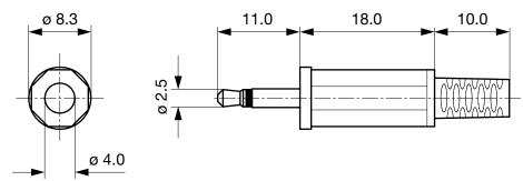
Cable diameter max. 4.0 mm
