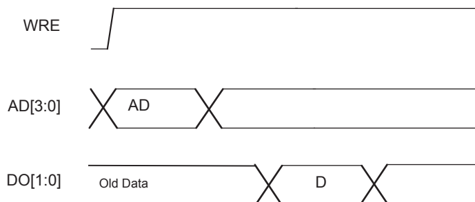
Figure 3-7. Slice Single /Dual Port Read Cycle Timing
