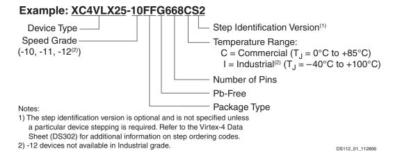
Figure 1: Virtex-4 FPGA Ordering Information
