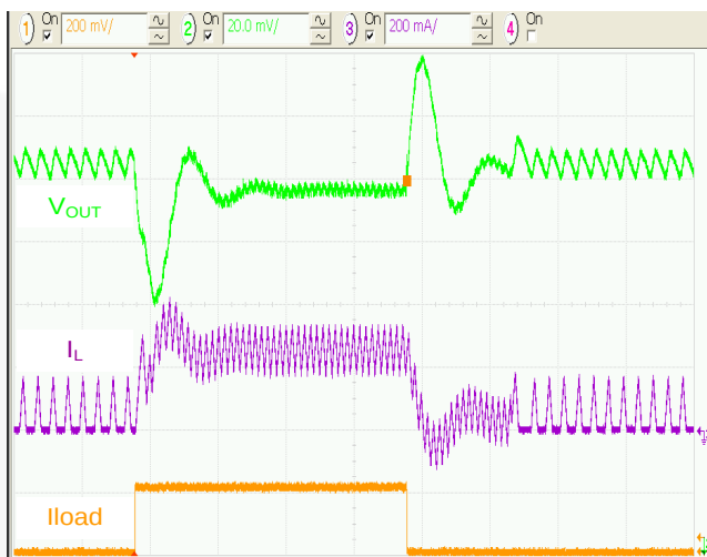
Figure 14. Load Transient 50 to 250mA, 3.6VIN, 5µs/div.
