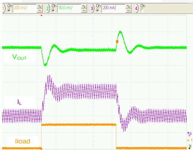
Figure 15. Load Transient 200 to 500mA, 3.6VIN, 5µs/div.
