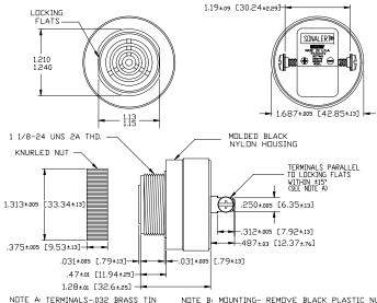
NOTE A: TERMINALS-032 BRASS TIN PLATED, TAPPED FOR #6-32 SCREW. TWO #6-32 NICKEL PLATED BRASS SCREWS INCLUDED. WILL ACCEPT 1/4\* QUICK CONNECT. E B: MOUNTING- REMOVE BLACK PLASTIC NUT AND INSERT THREADED FROM THROUGH 1.25' HOLE PUNCHED IN PANEL, IF DRIENTATION IS NEEDED, NOTE LOCKING FLATS ON DRAWING, SCREW NUT BACK ON. DD NOT OVERTIGHTEN.
