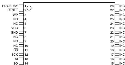
TSOP Top View Type 1
