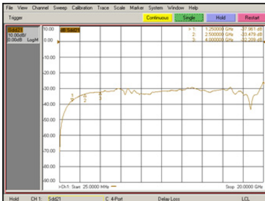
Fig 4. Differential Crosstalk – Super Speed
