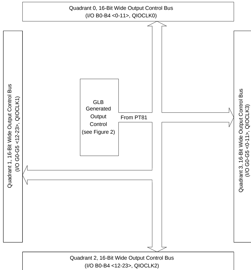
Figure 5. Output Control Bus and Quadrant Organization
