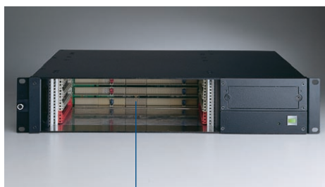
4-slot backplane with H.110 CT Bus
