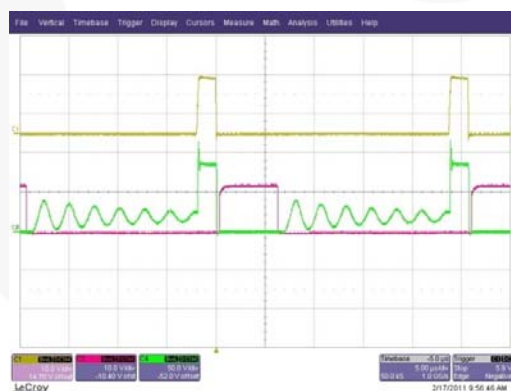
Figure 12. FAN6754AMR+FAN6204MY 230V/50Hz, 20% Load (Ch1: Gate, Ch2: Gate SR , Ch4: V dS )
