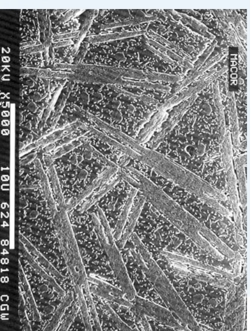
Microstructure of MACOR MGC. 5000X magnification.
