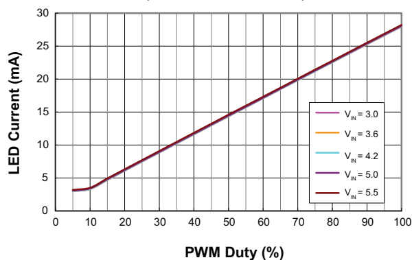
PWM Duty vs LED Current (AAT2893-2 10 WLEDs)
