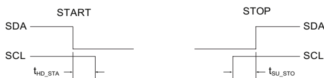
Figure 2: I²C STOP and START Conditions; START: A High "1" to Low "0" Transition on the SDA Line While SCL is High "1" STOP: A Low "0" to High "1" Transition on the SDA Line While SCL is High "1".
