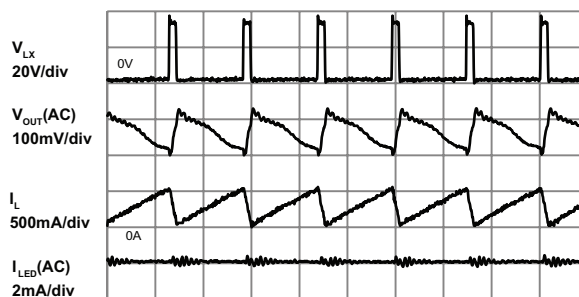
Switching Operation (AAT2893-1, V_{IN} = 3.6V , I_{LED} = 19.8mA , 10 WLEDs)
