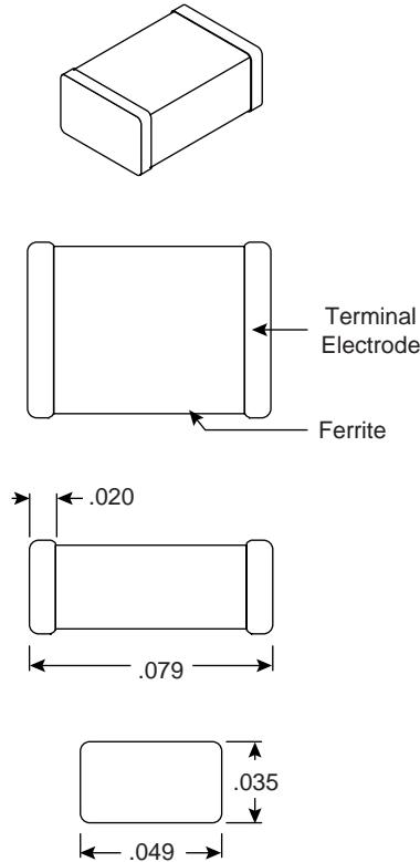
Ferrite Chip Beads provide an effective means of EMI/RFI attenuation for electronic equipment. These items are specially designed for flow, reflow, and wave soldering applications.
