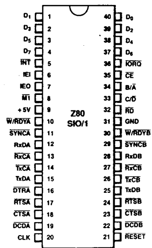
Figure 4. 40-pin Dual-In-Line Package (DIP), Pin Assignments
