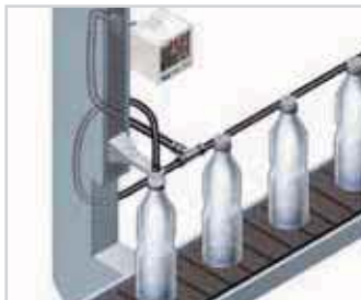
Air-leak test for PET bottles
