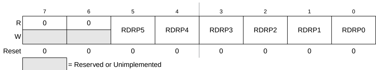
Figure 3-20. Port P Reduced Drive Register (RDRP)
