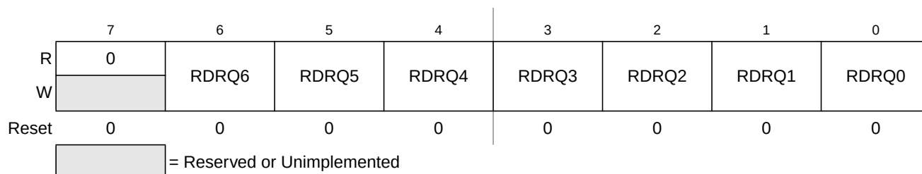
Figure 3-26. Port Q Reduced Drive Register (RDRQ)
