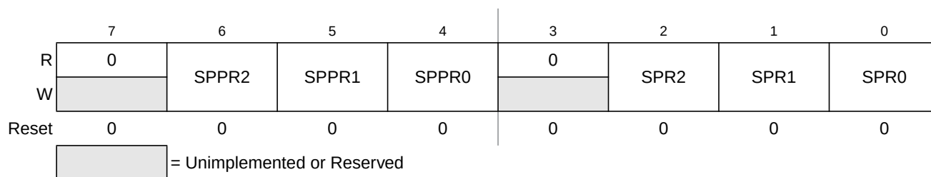
Figure 9-5. SPI Baud Rate Register (SPIBR)
