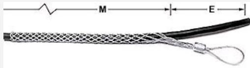
Slack Pulling Grips are offered in three styles made of galvanized steel. The closed type is used when the cable end is accessible. When not, there are split lace and split rod closing styles.
