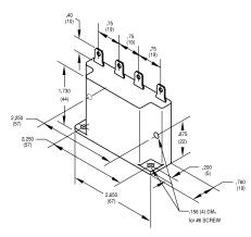
Operating Mode: Type 1: On-Delay. VTM-1 in-line timing module is wired in series with the load circuit. Time delay is initiated when power is applied to the series network. Connecting a resistor across the center terminals provides tamper-proof setting of time delay from 1-1000 seconds
