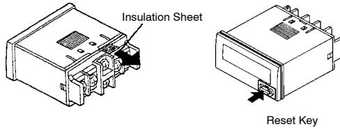
Switch settings on the Counter must be performed before mounting it to a control panel.
