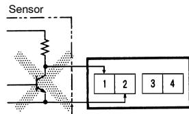
The operation of the Counter may be affected if the line voltage of the power supply exceeds 500 pF (about 10 m, with parallel wires of 2 x 2 mm). Keep all wires as short as possible. When using shielded wire, stray capacitance may occur.
