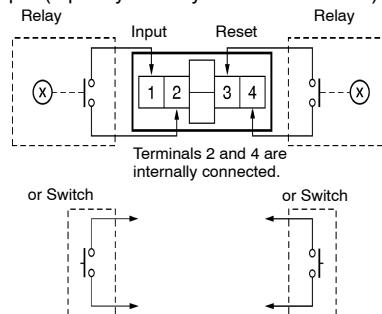
Note: Use Relays and Switches that have high contact reliability because the current flowing from terminals 1 or 3 is as small as approx.  $10 \mu\text{A}$ . OMRON's G3TA-IA/ID is recommended as the SSR.
