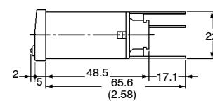
The wire-wrap terminals have a cross sectional dimension of 1x1 mm. Select one of three guages of wire from the table at right. Also listed in the table is the appropriate wiring hardware
