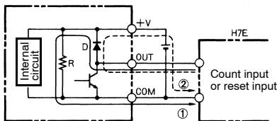
If an excessive voltage is applied to the count or reset input terminals, the internal elements may be damaged.
