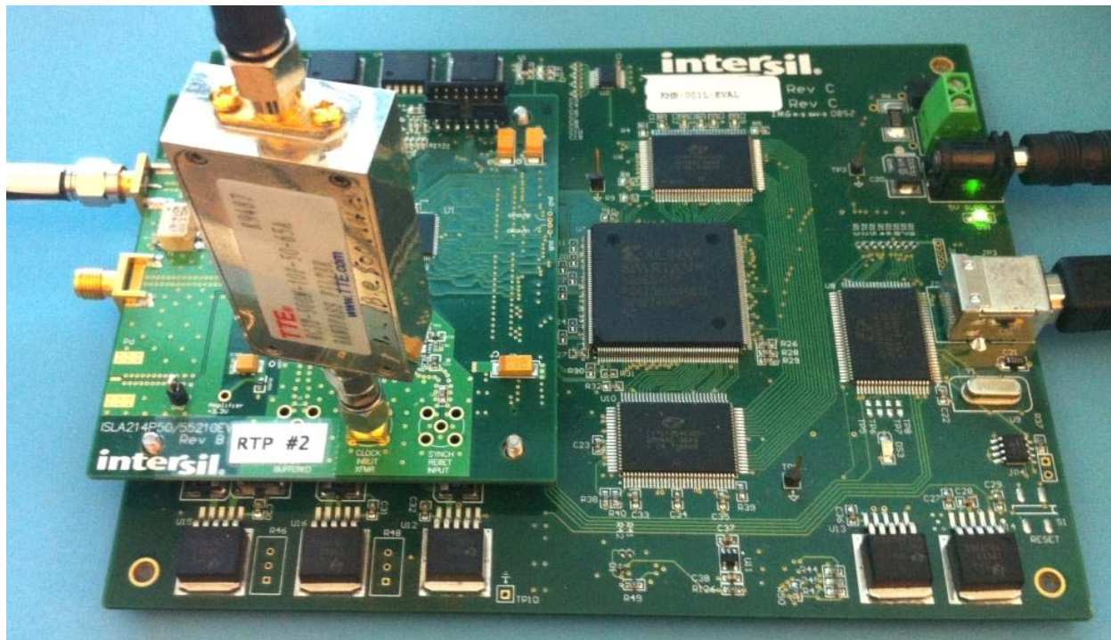
FIGURE 3. ISLA214P50-55210EV1Z DAUGHTERBOARD ON KMB-001 MOTHERBOARD
