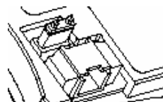
Figure 7: Slave Setting for Vertical iDiskOnChip 40-Pin Connector
