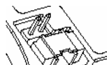
Figure 9: Master Setting for Vertical iDiskOnChip 40-Pin Connector
