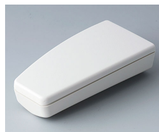
A9066107 SMART-CASE M, Vers. I ABS (UL 94 HB) off-white RAL 9002 3.78"x1.85"x0.94" IP 40
