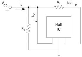
The resistors  $\rm R_b$  and  $\rm R_L$  can be used to bias the input current, lin. Refer to the part specification for limiting values. This circuit will help in getting the precise ON and OFF currents desired.
