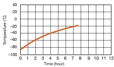
Pull-up characteristics during power failure
