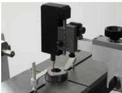
Checking of small plain ring gages from Ø 2 mm as standard
