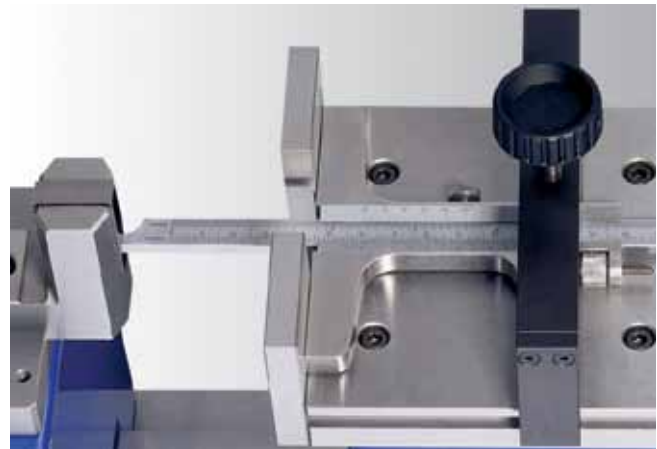
▲ Checking of depth calipers using gage block anvils (54-190-805) & depth gage attachment (54-190-827)
