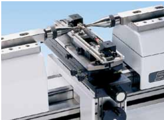
▲ Checking of plug gages and threaded plug gages from dia. 1.18" to 10"/30 to 250mm using table (54-197-011), clamps (54-197-142), small Ø anvils (54-190-806) & thread wires (54-197-007)
