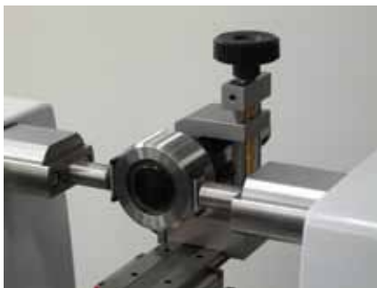
Checking of thread plug gages
