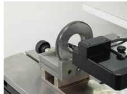
Checking of taper thread ring gages
