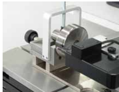
Checking of taper thread plug gages
