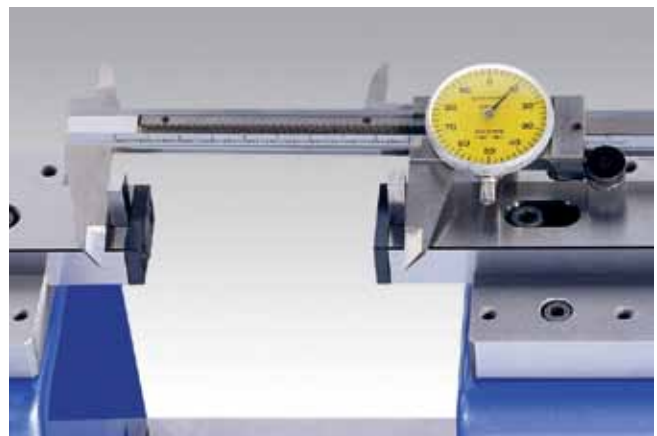
▲ Checking of calipers using 54-196-006
