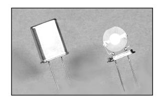
The MP Series are the right choice for Microprocessor, controller, or other standard crystal applications. These hermetic packages use Resistance Weld sealing for improved aging and reliability. Surface mount lead forming is available as well as insulating sleeve, top wire, bent leads, or tape/reel packaging.
