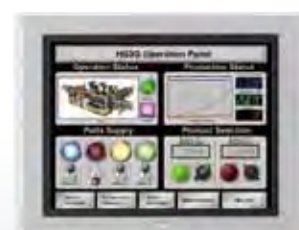
Photo: HG3G Operator Interface
