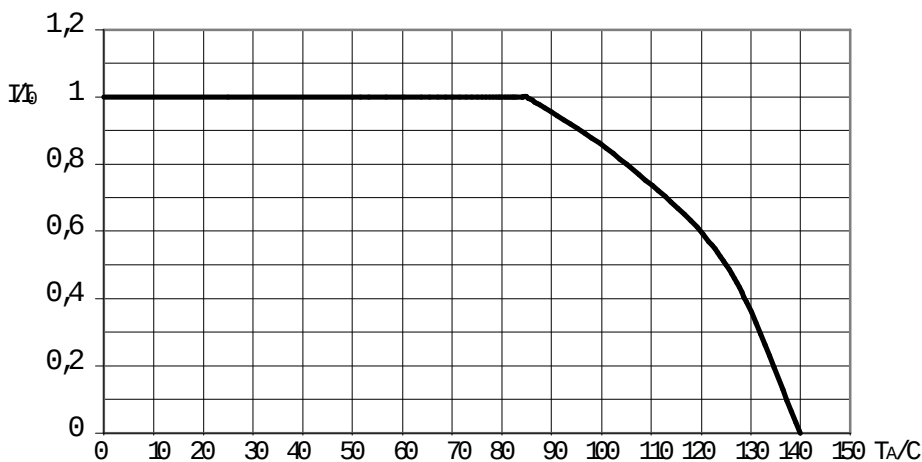
B82464-XXXX-X: current derating versus ambient temperature
