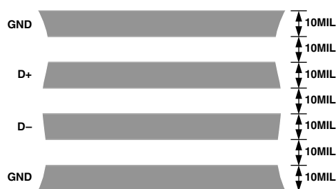
Figure 8. Arrangement of Signal Tracks
