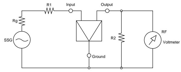
$R_g + R_1 = R_2$  : Input/Output Impedance
