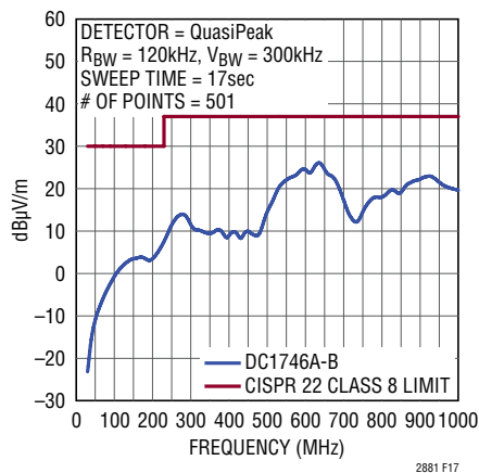
Figure 17. Low EMI Demo Board Emissions
