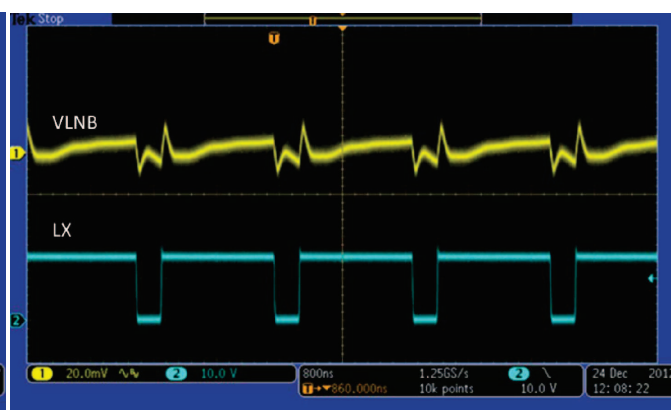
Figure 6. Boost LX Waveform at 0.5 A, ( V_{IN} = 12\text{ V} , V_{LNB} = 13.4\text{ V} )
