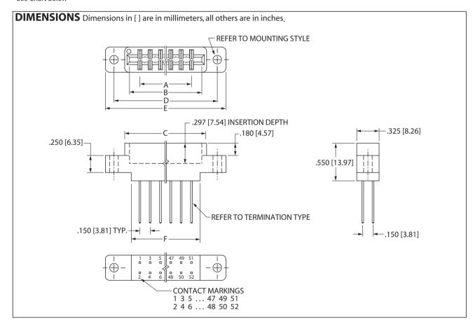
Tolerances on non-critical dimensions may very slightly due to shrinkage differential per insulator material; Consult factory.
