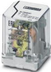
Plug-in high-power relay with power contacts, specifically for switching high DC loads, 1 N/O contact, blowout magnet, coil voltage: 230 V AC
