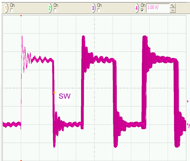
Figure 39. SW-Node Jitter (Infinite Persistence), I_{LOAD} = 200mA , 50ns/div.
