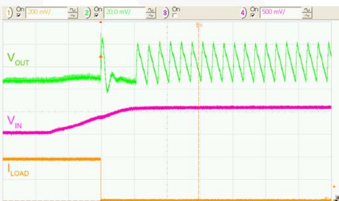
Figure 23. Combined Line/Load Transient 3.3 to 3.9V_{IN} Combined with 400mA to 40mA Load Transient
