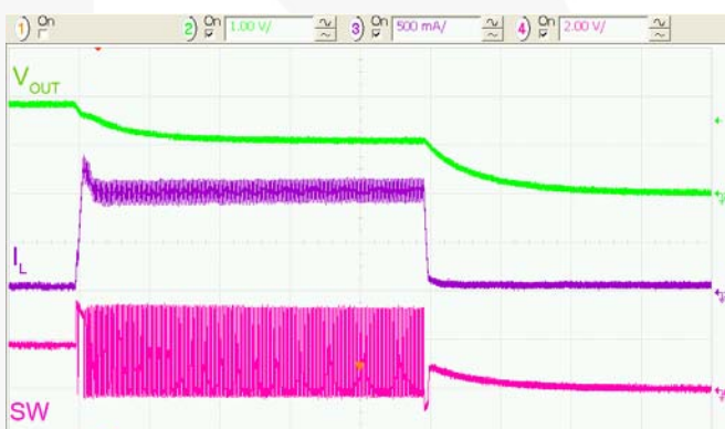
Figure 36. Over-Current Fault Response, R_{LOAD} = 1\Omega
