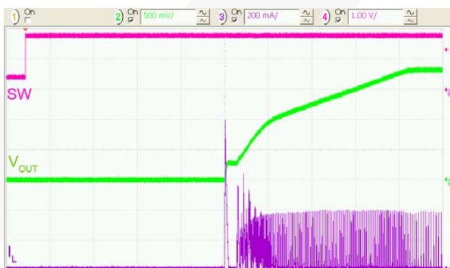
Figure 38. Soft-Start, R_{LOAD} = 50\Omega , 20\mu s/div.
