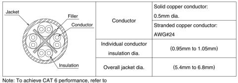
TM23P-88P Cable Termination Procedure Manual (ETAD-E2415).
