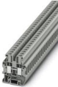
Mini feed-through terminal block, Connection method: Screw connection, Cross section: 0.2 mm<sup>2</sup> - 6 mm<sup>2</sup>, AWG: 24 - 10, Width: 6.2 mm, Color: gray, Mounting type: NS 15
