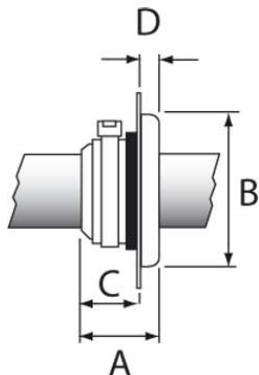
Material with high elasticity, supplied with one Ty-Rap® cable tie to ensure a stable, tight and sealed strain relief. Simple and quick installation. Typical applications: in control cabinets, in the building of motor vehicles, in the construction of machines,...
