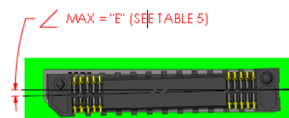
INITIAL Z AXIS ANGULAR MISALIGNMENT
