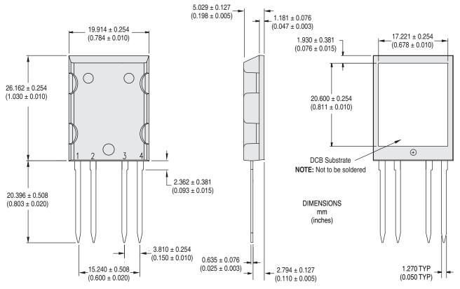
**NOTE:** Metallized external surface of DCB substrate maintains 2500V isolation to device internal structure and all external pins.
