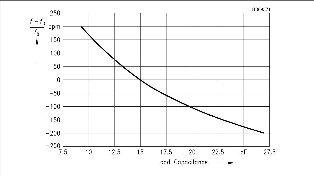
Figure 69 DCO2 Tuning Range (12.352 MHz Crystal) Crystal specified for C_L = 15 pF
