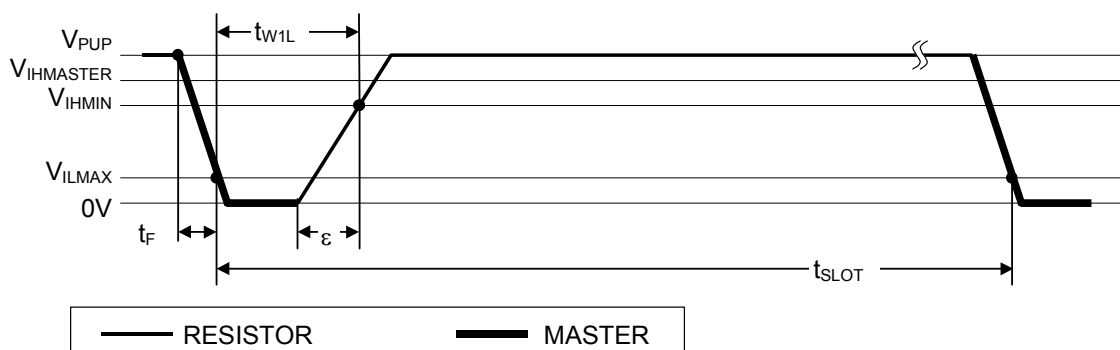
Figure 7. READ/WRITE TIMING DIAGRAM
